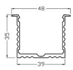
Can be used as a main lighting source. Especially designed to except 2 led strips.
