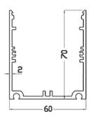
Suitable for two T5, T 8 Lighting tubes or Led Strips.
