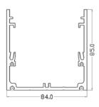
Suitable for two T5, T 8 Lighting tubes or Led Strips.
