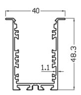
Suitable for one T5 Lighting tube or Led strips.
