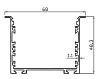
Suitable for two T5, T 8 Lighting tubes or Led Stips.
